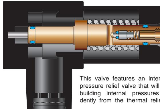
This valve features an internal safety pressure relief valve that will discharge building internal pressures independently from the thermal relief function
