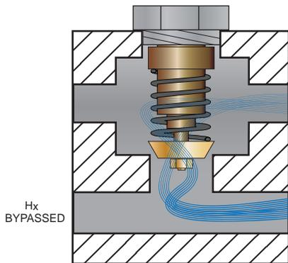
**Fig 1. VALVE STATE: OPENED** - THE VALVE WILL BYPASS THE COOLER WHEN THE FLUID IS COOL ENOUGH. PRESSURE DIFFERENTIAL BETWEEN THE COOLER AND THE BYPASS ENABLES THE BYPASS TO OCCUR WITHOUT ADDITIONAL COMPONENTS.
