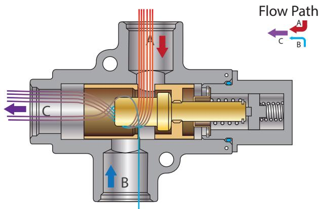
**Fig1:** Restricted cold flow into port B
