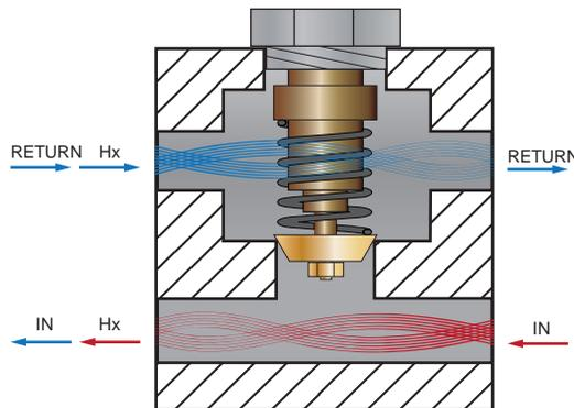
**Fig 2. VALVE STATE: CLOSED** - WHEN SYSTEM FLUID REQUIRES COOLING THE VALVE CLOSSES AUTOMATICALLY. FLUID MUST FLOW THROUGH THE COOLER WHEN THE VALVE IS CLOSED. THE CHILLED FLUID CROSSES OVER THE SENSING UNIT OF THE VALVE AND OUT INTO THE SYSTEM.
