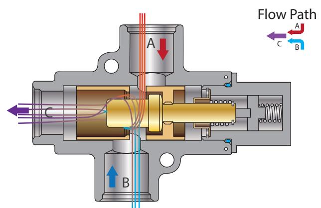
**Fig2:** 50 / 50 mix between hot and cold inputs
