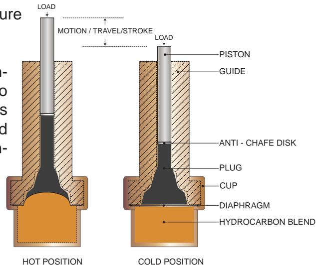
The expansion/contraction of these thermal actuators can be utilized to operate a valve, mechanical linkage, electric switch, or any other device. The plug and diaphragm type are proven to be the most reliable style for any application.
