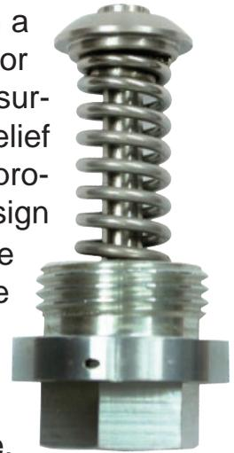
As fluid is diverted, the pressure inside the vessel drops. Once the internal forces reach the valve's re-seating pressure the valve will close. The blowdown is usually stated as a percentage of set pressure and refers to how much the pressure needs to drop before the valve re-seats. The blowdown can vary from roughly 2-20%, and some valves have adjustable blowdowns.
