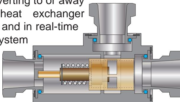
Figure 2. Valve cross-section shown in "hot" position
